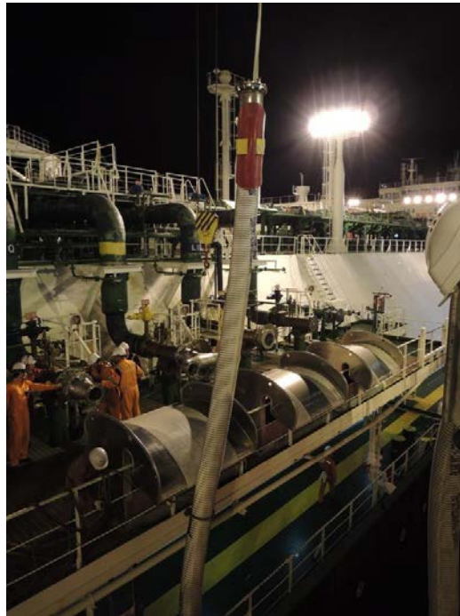
Figure 20 – Hose is being secured with 25 mm rope
