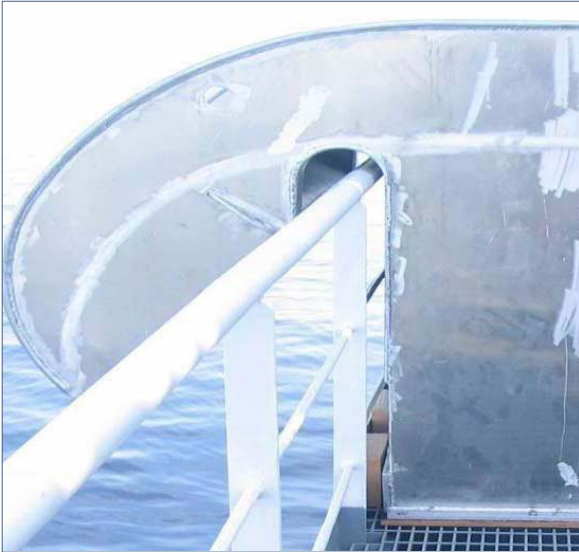
Figure 17 - Correctly positioned saddle
