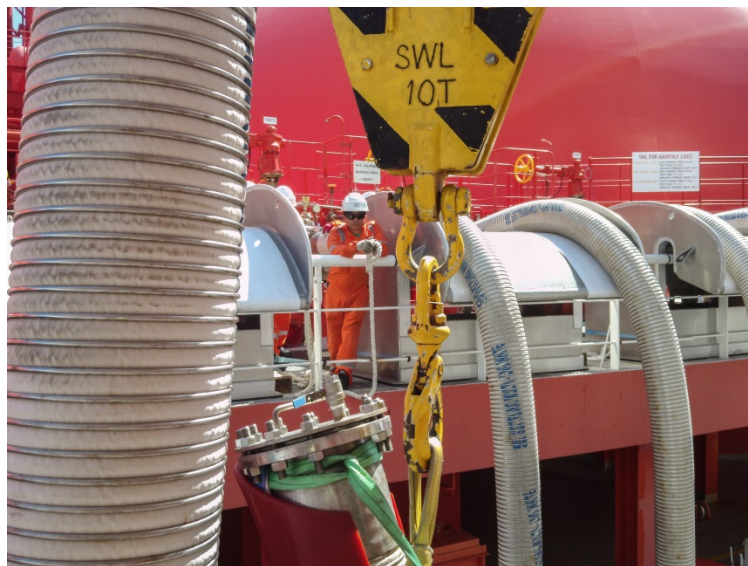
Figure 18 - Transfer of hose from FSRU to LNGC
