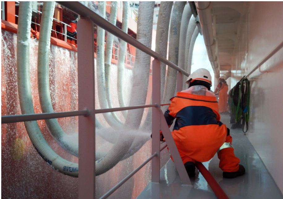
Figure 22 - Liquid freeing of cargo hoses
