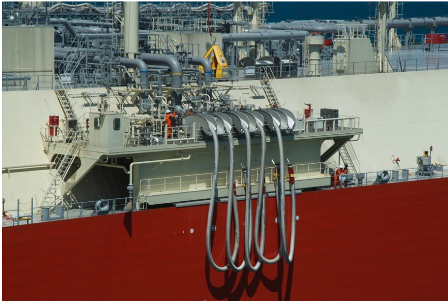
Figure 16 - Stowage position of cargo hoses
